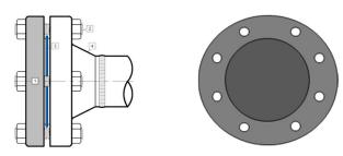
Pancake Blind - a blind that is temporary inserted between two flange faces in a line to block the flow. The blind has a handle that is used to insert and remove the blind. This blind is also referred to as a skillet blind, slip blind, spade blind, or a fan tail blind.
