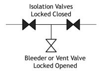
**Double Isolation** - the isolation of a line, duct or pipe by closing and locking out a single in-line valve, installing a slip blind, and opening and locking a drain or vent valve in line between the valve and the slip blind.
