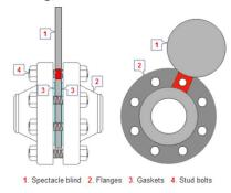
Blind Flange - a plate for covering or closing the end of a pipe.
